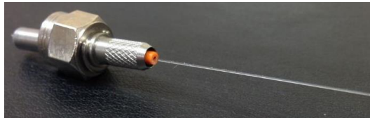
Figure 4: Ce 3+ doped SiO 2 fiber
