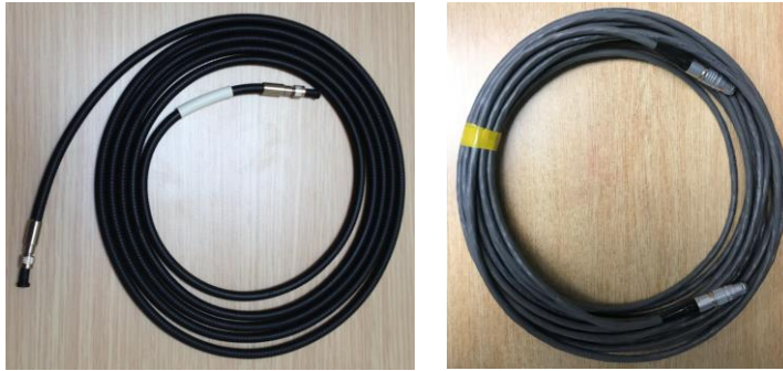
Figure 6: Fiber optic cable, 400 \mu , 15m (Left) and motor cable, 15m (Right)
