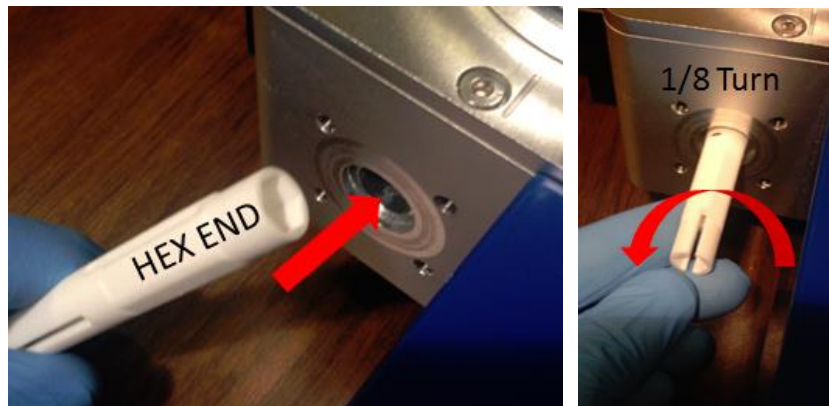
Figure 33: Insert hex-socket of empty cartridge to loosen fiber 1/8 turn.
